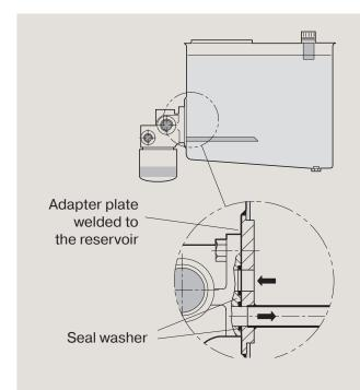
Fig. 5. Boost unit/reservoir installation (example).
