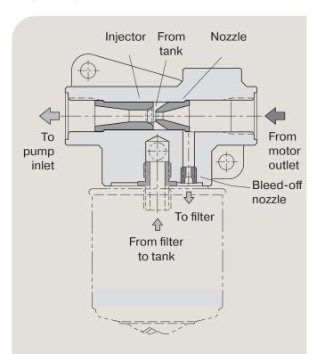
Fig. 1. BLA boost unit cross section.
