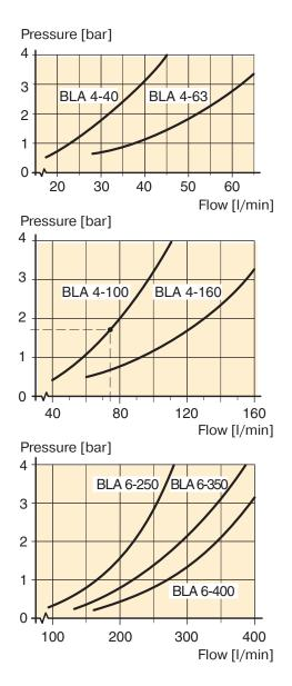
Fig. 4. BLA pressure/flow diagrams.
