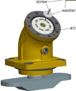
2. Fasten screw and washer to secure that the cylinder barrel (item 411) stays in correct position.
