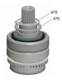
7. Disassemble the retaining ring (item 478) and the spacer washer (item 476).
