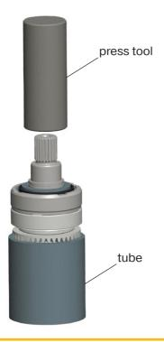
8. Place the bearing package on a tube and disassemble the bearings by pressing on the shaft end.
