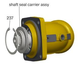
18. Assemble shaft seal carrier assy by using a tube. Carefully tap it in with a hammer.
