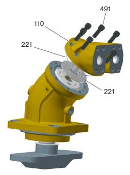
22. Assemble the valve plate (item 121) in the end cap (item 110), use some grease to keep it in position. Place the O-ring (item 221) on the end cap (item 110).
