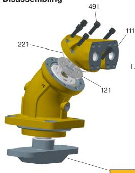
1. Fasten the fixture in a vise and place the motor in the fixture. Loosen the bolts (item 491). Carefully remove the end cap (item 110) and the O-ring (item 221). Make sure the valve plate (item 121) don't fall out.
