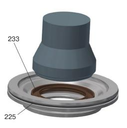
17. Assemble the shaft seal (item 233) and O-ring (item 225).
