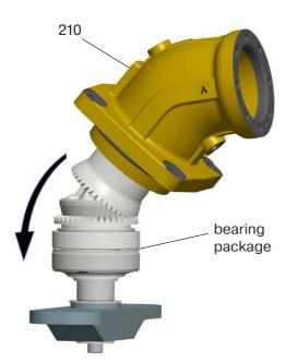
15. Carefully place the bearing housing (item 210) on the bearing package.
