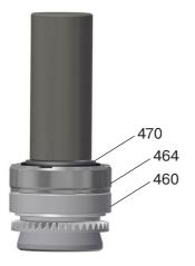
11. Place the spacer ring (item 464) and the tappered roller bearing (item 470) on the shaft.
