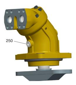
24. Assemble hexagon plug (item 250) according to customers specification.
